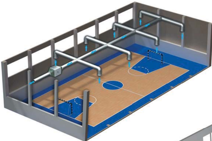
VS fan gym ventilation example
